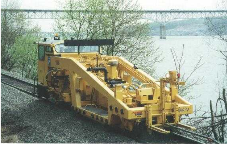
Example of one of many types of machines I have been involved in the design of. This is a Tamper, and it is used to surface and align railway track work.
