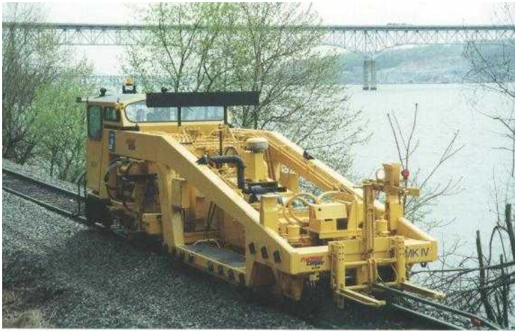
Example of one of many types of machines I have been involved in the design of. This is a Tamper, and it is used to smooth and align railway track. It is a complex structural machine using Diesel power and computer controlled hydraulics to control the machine and do the work.
